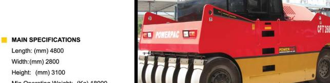
Min Operating Weight: (Kg) 18000 Max Operating Weight: (Kg) 26000
